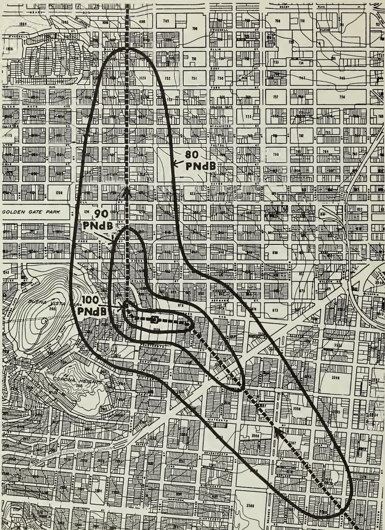
FIGURE IV-8 PERCEIVED NOISE LEVEL (PNdB) CONTOURS FOR LANDING AND TAKEOFF OF LIGHT OR MEDIUM WEIGHT TURBINE POWERED HELICOPTER
